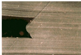
Figure 4b - Microscopic View of Smooth Edge Welding Revealing Void-free Fusion and Transition
