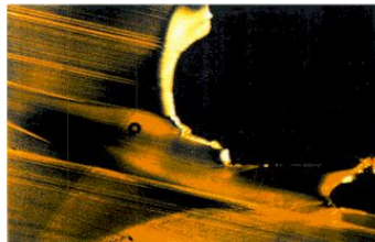
Figure 2 - Microscopic View of Torn Hot Wedge Flap Showing Ductile Tear and Several Points of Cracking Caused by the Tearing Action
